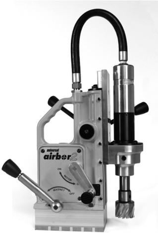
Re-check the unit is correctly positioned for the hole to be cut, and close the magnet handle extension.
